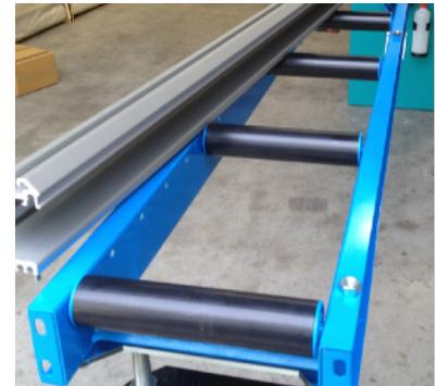
3. Drill additional holes spaced at about 1m to 1.5m apart into the top rear lip of the roller conveyor frame (where the measuring stop will be mounted).
