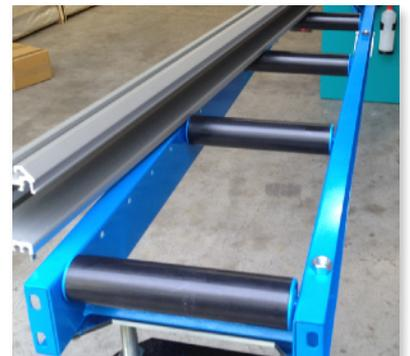
3. Drill additional holes spaced at about 1m to 1.5m apart into the top rear lip of the roller conveyor frame (where the measuring stop will be mounted).
